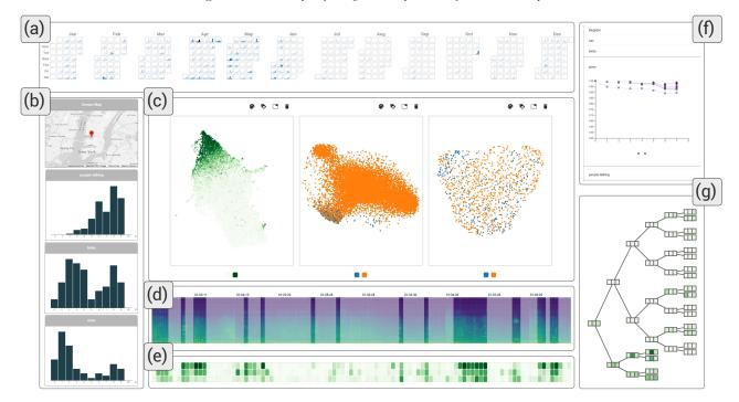
**Figure 3:** The Urban Rhapsody system visual interface: (a) Calendar View; (b) Sensor Map and Distribution View; (c) Day View (projections); (d) Focused View (spectrograms); (e) Frame Classification View; (f) Model Summary; (g) Mixture Explorer.
